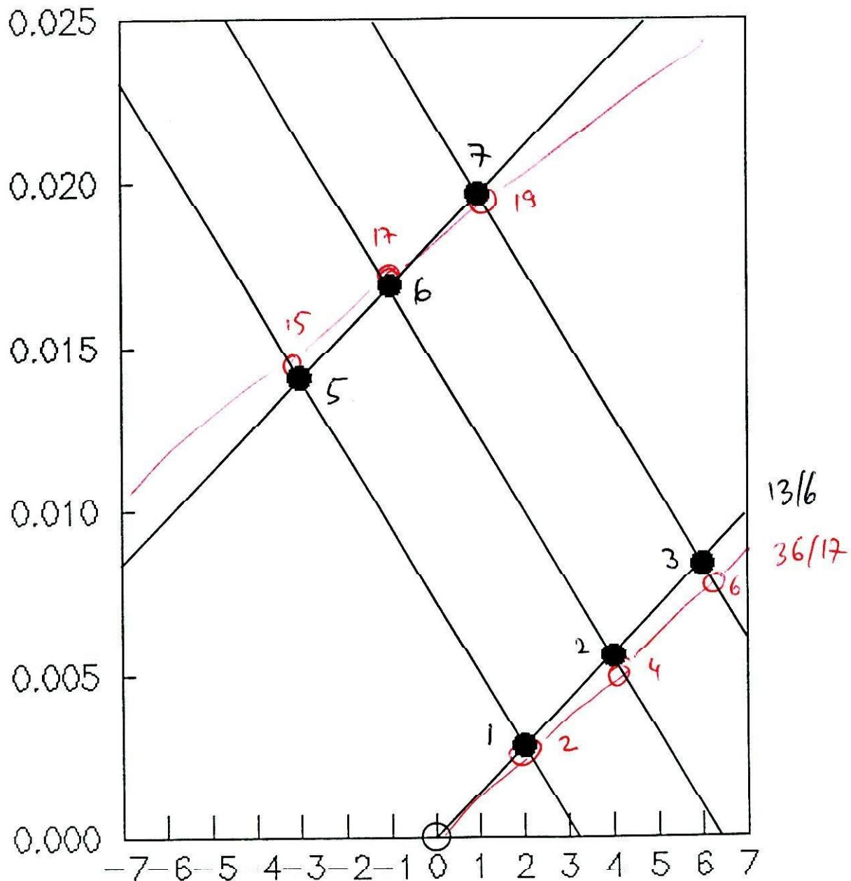
Interpretation: Although the fractional indexing produces widely different indices, the expected diffraction spots and layer lines have moved only little, as can be expected from the similar geometry.
