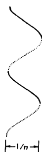
Fig. 7.40 The projection of a thin helix, as in Fig. 7.39a. It is left-handed, and its upper surface (whose projection gives the F.T. shown in Fig. 7.42) is drawn as a continuous line. The diameter is 1/\pi so that Fig. 7.41 shows, with the correct scale, the F.T. of both surfaces.
