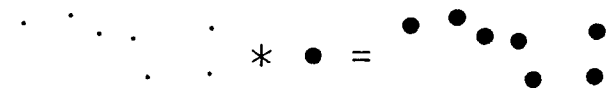
Fig. 7.13 A series of points arranged in the pattern of a familiar stellar constellation is convoluted (*) with a circle. This replaces each point by a copy of the circle.
