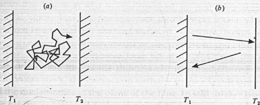
Fig. 31. Principle of thermal conduction by laminar (a) and molecular (b) conduction between the surfaces at temperature T_1 and T_2 .
